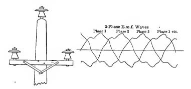
FIG. 45. Three-phase transmission line and diagram of e.m.f. waves in the three circuits.
